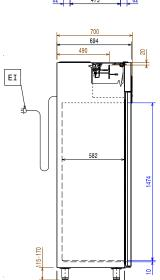
**EI** = Electrical inlet (power) Refrigerant Inlet R0 = Refrigerant Outlet
